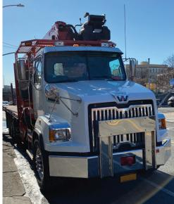
2015 Western Star with 92 ft Fassi F390 Crane, Dump Bed and 25" Grapple Saw
